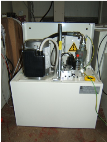
IGV pump unit which uses a standard triangular lift key
