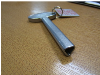
IGV pump unit which uses a standard triangular lift key
