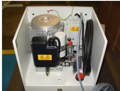
RFP unit that uses a cylindrical key. Stannah part no. : 556054
